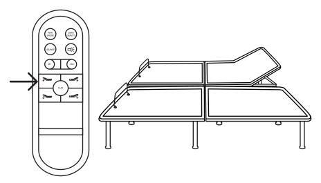
**10** To Toggle between Flex-Head Mode and Standard Mode, press and hold both the "Anti-Snore" & "Zero Gravity" simultaneously on the remote until you hear one or two beeps. One beep means you are in Flex-head mode, two beeps means you are in Standard Mode.
