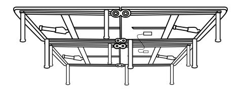
**9** Use one of the two remotes and press the head up button. If both heads rise, the base is in Standard Queen Mode. If only one rises, the base is in Flex-Head Mode.
