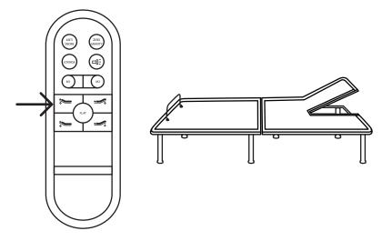
**8** To Toggle between Flex-Head Mode and Standard Mode, press and hold both the "Anti-Snore" & "Zero Gravity" simultaneously on the remote until you hear one or two beeps. One beep means you are in Flex-head mode, two beeps means you are in Standard Mode.
